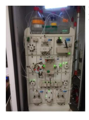
The PETC has a Bio-Rad NGC and Bio-Rad DuoFlow chromatography systems for low to medium pressure chromatography. Both are kept at 4°C.
