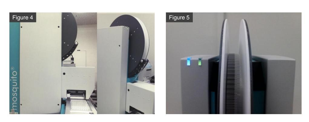
A TTP LabTech Mosquito Crystal nanodispenser (Figures 4 and 5) was used to setup the tray in under four minutes after the loading plates were prepared manually. A Greiner V-bottom 651101 plate was used to hold a protein dilution (Column 7) row A-H, the seed stock in a separate column (Column 8), and water to wash the seed in four additional columns. The loading plate is detailed in Table 1.
