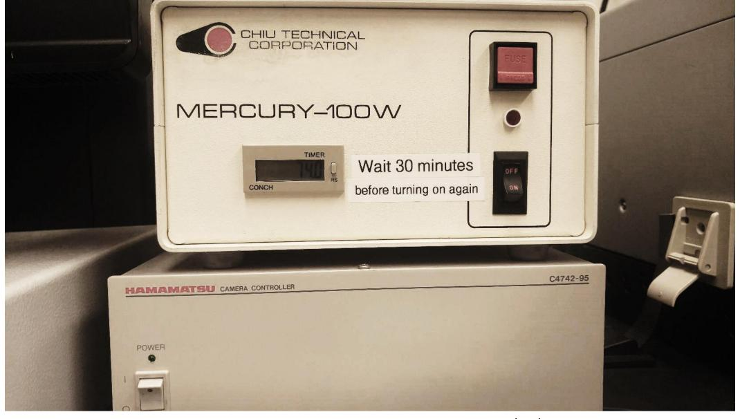
THE MERCURY BULB POWER SUPPLY AND HAMAMATSU (UV) CAMERA CONTROLLER SHOULD BE IN THE OFF POSITION. LOOK TO SEE HOW MANY HOURS ARE ON THE TIMER. THESE ARE LAMP HOURS.
